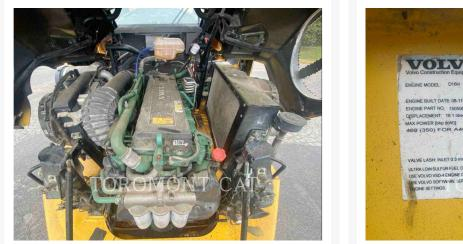
VOLVO ON CONTROL INFO ABEL ENGINE BUILT DATE VETT ENGINE PART NO. 1505068 DISPLACEMENT: 16.1 litres MAX POWER [bhp (kW)] 469 (350) FOR A40 DUPLICATE VOLVO WORK INCOMENTATION ON THE STATE ONLY, MAX 15 PPM S VIO VSD-4 ENGINE OIL, OR EQUIVALENT VIO SOFTWARE SERVICE TO DUT O VER SETTINGS. - Van
